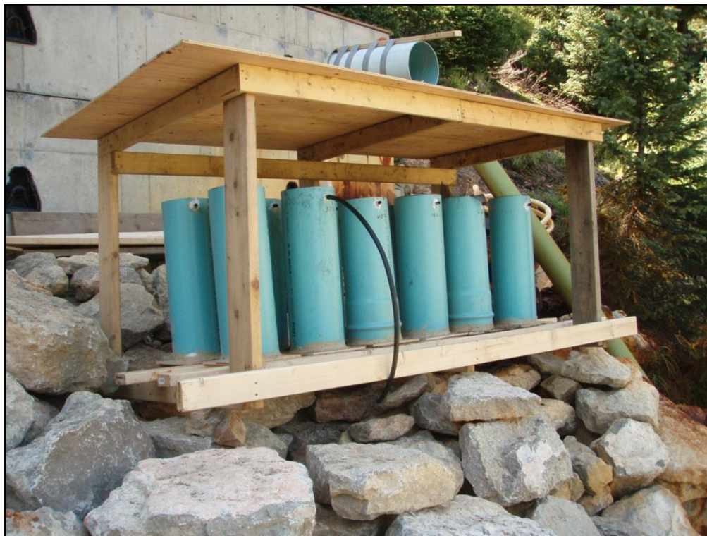
Figure 29. Column experiment at the Eveline Mine.
