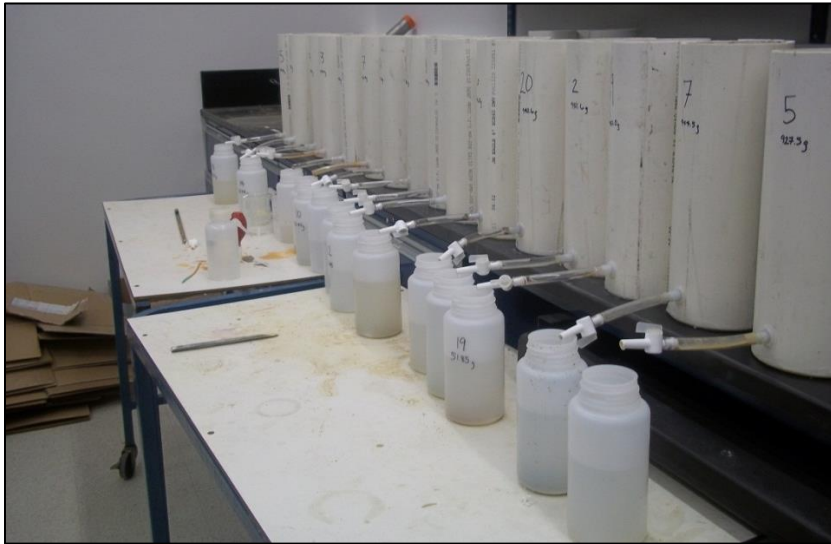
Figure 85. USGS laboratory set-up for soil column experiments.
